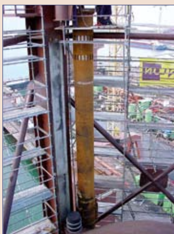
The generator floaters can be slowed down by four water brakes, each of which consists of two pipes sliding one inside the other, with one of the pipes moving up and down with the floater. The braking power can be adjusted by means of a hydraulically controlled valve through which the water is expelled.
