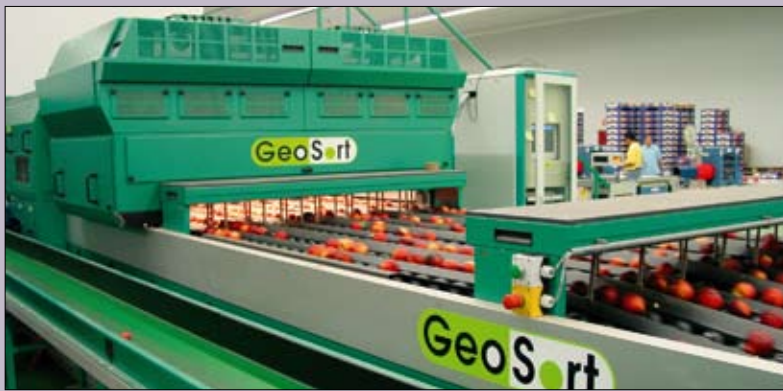
Sorting machine for apples and other types of fruit, manufactured by Greefa BV, Tricht. Image processing plays a major role in the sorting process. (Photo: Greefa BV, Tricht)
